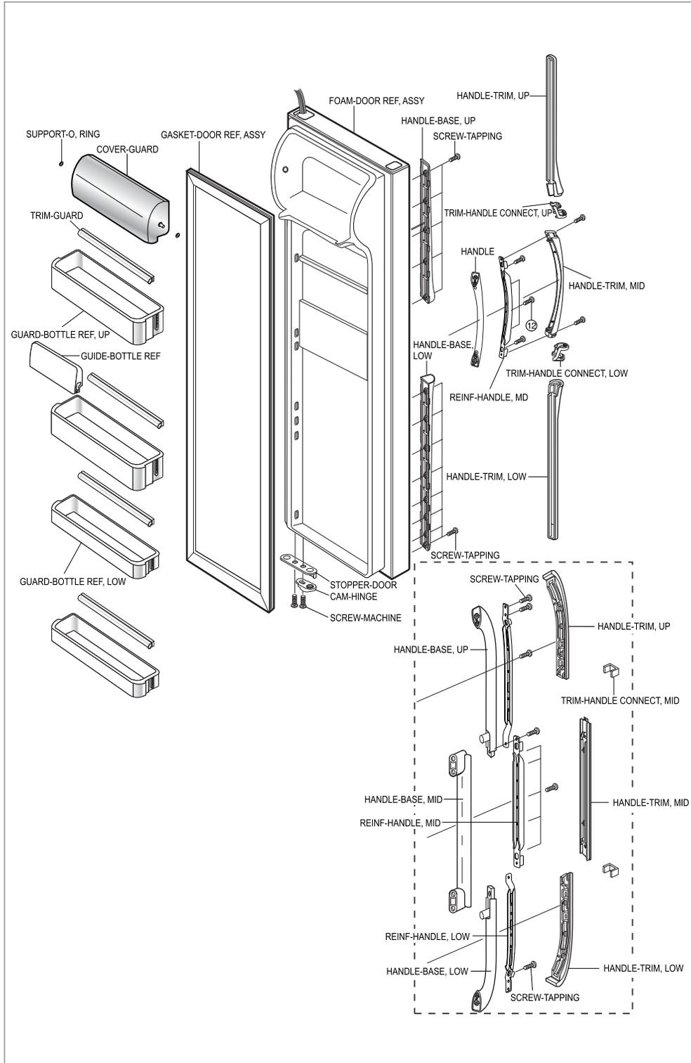
14-7) Freezer Room Door Exploded View (SR-S2028, S2029, S2228, S2229/S20DTC, S20FTC, S22DTC, S22FTC)
