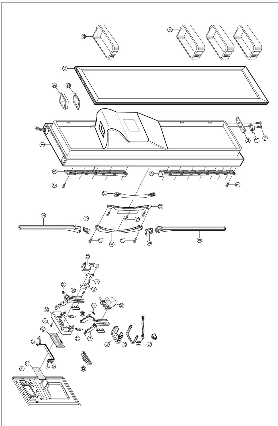
14-8) Refrigerator Room Door Exploded View (SR-S2027,S2029, S2227,S2229/S20FTC,S22BTC,S22FTC)
