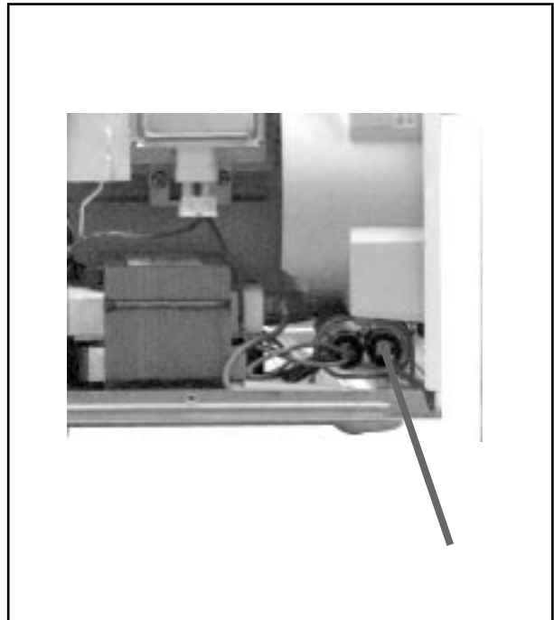
Fig. 1-1. Discharging the High Voltage Capacitor
